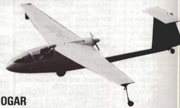
Two-seater Training Motor Glider Limbach Pusher engine 68 HP Glide angle 1:27 supplied with full set of instruments. Demonstrator at Lasham from end of JUNE
