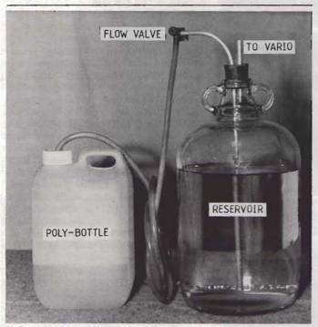
Fig 1. The assembled calibrator.
