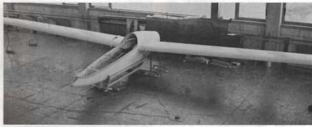
Development work on the DG-500. The wings assembled to a fuselage part for moulding the wing fuselage fairings.
