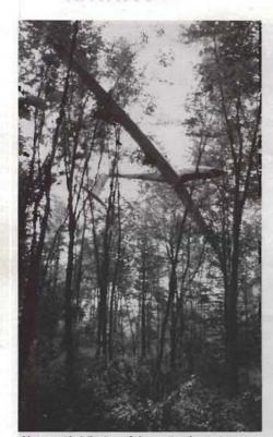
Above and at the top of the next column, two ASW-20s after a mid-air collision during the 1984 Open Class Nationals at Lasham. The crowded situation near the gate and startline of a competition carries a higher risk than usual but most collisions take place between the only two aircraft in the vicinity.
