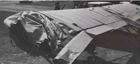
Damaged Super Cub after a collision with a Nimbus 2.
